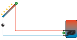
Internal heat exchanger, intelligent pump control
